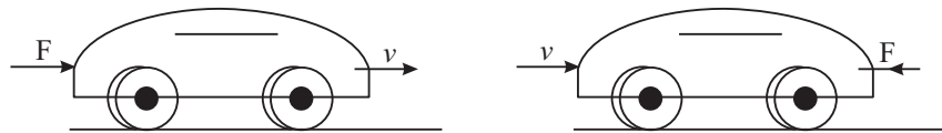
Fig. 6.2 : A car is moving on a horizontal road. a) A force F is applied in the direction of the moving car. It gets accelerated. b) A force F is applied in opposite direction so that the car comes to rest after some distance.
