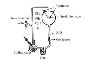
Fig.1.2 The apparatus used by Stanley Miller and Harold C. Urey to demonstrate the synthesis of amino acids under conditions that existed on the primitive earth
