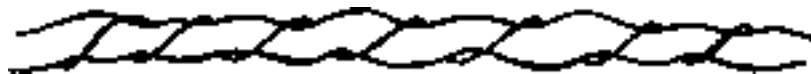
Fig. 23.8: (b) SPIRA or GIMP- combination of soft, thick yarns twisted with fine, hard yarns
