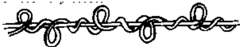
Fig. 23.8: (d) LOOP – stiff fibres form loops which spring out of the core yarn
