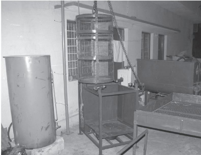
Fig. 4.4: Indigenous arrangement for removing water from straw. Mechanism is like washing machine. Motor below, container for straw on top
