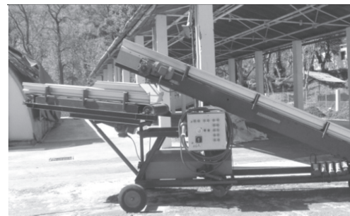
Conveyer with front moving head for tunnel filling
