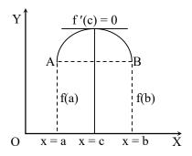
The theorem states that between two points with equal ordinates on the graph of f, there exists at least one point where the tangent is parallel to x-axis.
