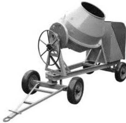
**Fig. 10.2:** Concrete Mixer for use at site
