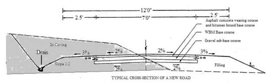
Fig. 17.1: A typical cross section of the road
