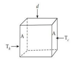
Thermal conductivity of a material is defined as the amount of heat transferred in one second across a piece of the material having area of cross-section  $1m^2$ and edge 1m when its opposite faces are maintained at a temperature difference of 1 K. The SI unit of thermal conductivity is W m<sup>-1</sup>k<sup>-1</sup>
