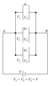
equivalent capacitance of a number of capacitors joined in parallel is equal to the sum of the individual capacitances. Remember that in parallel combination, all the capacitors have the same potential difference between their plates but charge is distributed in proportion to their capacitances
