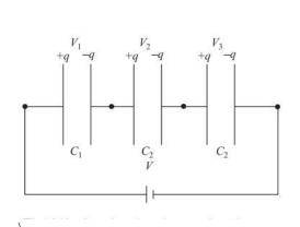
The second plate of the first capacitor is connected to the first plate of the second capacitor. The second plate of second capacitor is connected to first plate of the next capacitor of the combination and so on. The second plate of last capacitor of the combination is connected to the electrical source
