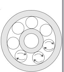
Fig. 3.6 : Balls in the ball-bearing
