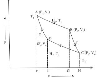
Fig. 11.4 : Indicator diagram of Carnot cycle
