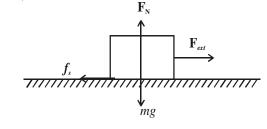
Fig. 3.4 : Forces acting on the block
