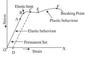
Fig. 8.9: Stress-strain curve for a steel wire
