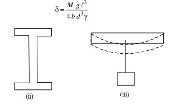
Thus for a given load, we will select a material with a large Young's modulus Y and again a large thickness to keep  $\delta$  small. However, a deep beam may have a tendency to buckle (Fig iv). To avoid this, a large load bearing surface is provided. In the form I-shaped cross-section, both these requirements are fulfilled.
