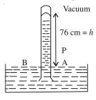
Fig: 9.6 : Toricelli's Barometer
