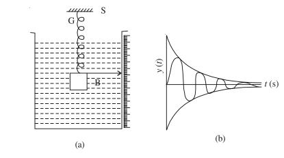
Fig. 13.14 : Damped vibrations : (a) experimental setup; (b) graphical representation
