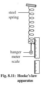
You should know that the materials which obey Hooke's law are used in spring balances or as force measurer, as shown in the Fig. 8.11. You would have seen that when some object is placed on the pan, the length of the spring increases. This increase in length shown by the pointer on the scale can be treated as a measure of the increase in force (i.e., load applied).
