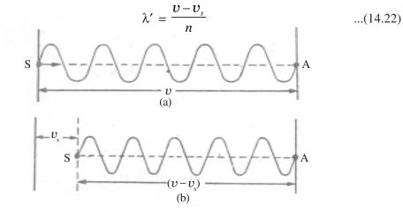
Fig. 14.18 : Crowding of waves when source is moving
