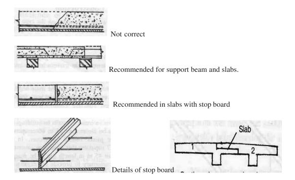
Fig. 10.6: Construction Joints
