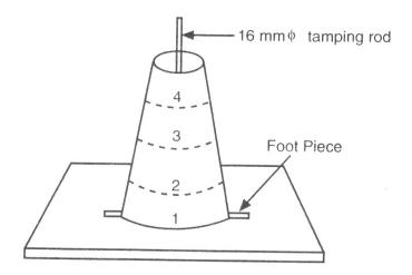
**Fig. 10.7:** Slump test (step 2)
