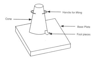
Fig. 10.7: Slump test (Step-1)
