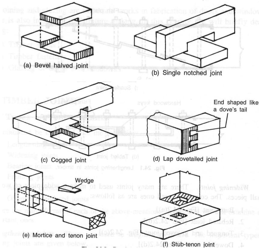
**Fig. 15.10:** Joints used in the wooden works.
