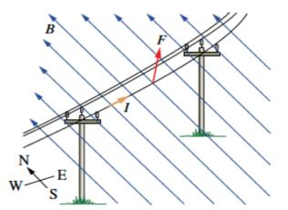
Calculate the magnitude of the force due to the earth's magnetic field that acts on this suspended power line carrying a current of 100 A from west to east. Assume that the earth's magnetic field at this point is  $5.0 \times 10^{-5}$  T.
