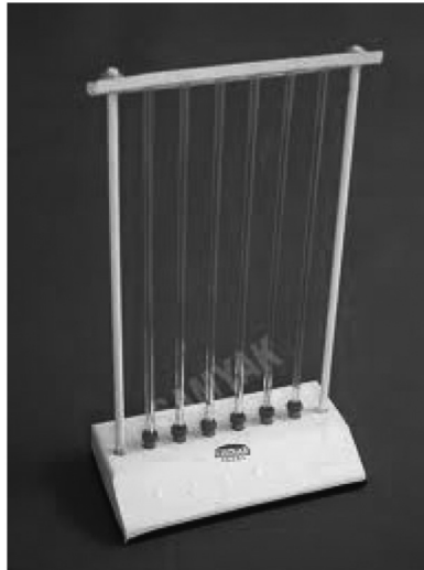
Fig. 8.2: Westergren pipette filled with blood and placed vertically on the rubber cork in the rack
